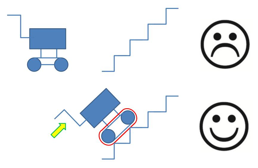
Switch between four-wheel and chain-drive of the vehicle under actual conditions (by pushing a button)
